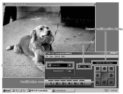
The connected VN-C2U angle steps of the pan/tilt can be changed using the right and left arrow buttons ( $\square$  and  $\square$ ).
